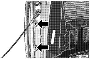
2. Pull the housing straight out from the body, with a quick motion, to separate the housing from the body. If not pulled straight, locators may be damaged.
